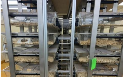
ColonyRack that allows any mouse to access any cage on the rack
